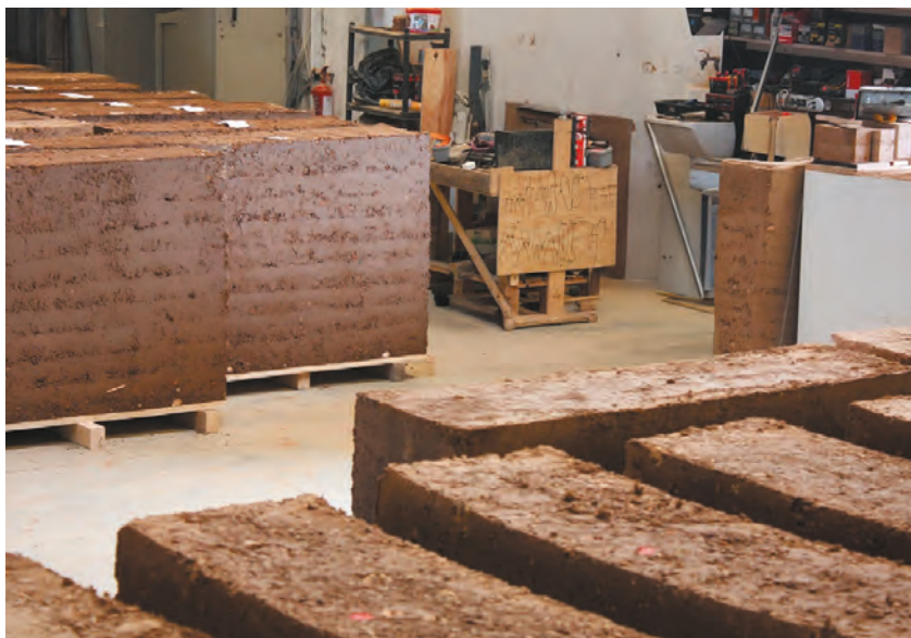
Workshop of the start-up Terrio, specialising in the manufacture of compressed earth building materials.
